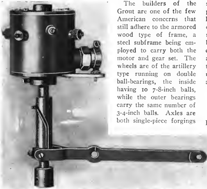
Grout Synchronous High Tension Distributor Showing Advance.
